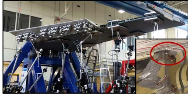
Test article (ILEF lugs)
